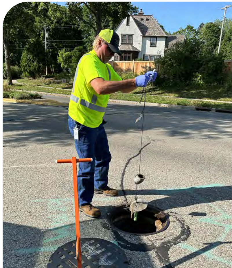
Collection system supervisor Ray Schneider collects wastewater samples for COVID variant testing in the service area.
